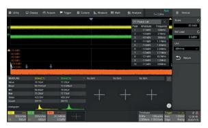
T3DSO3204: At 200 MHz bandwidth, the input noise floor is typically only 80 uVrms.
