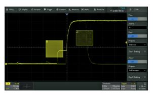
Set up to 2 zones defining each as either an Intersect or a Non Intersect. Trigger occurs when conditions are met. Zone Trigger helps to simplify advanced triggering.
