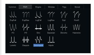
The 25 MHz function / arbitrary waveform generator comprises 6 standard waveforms and 45 arbitrary waveforms.
