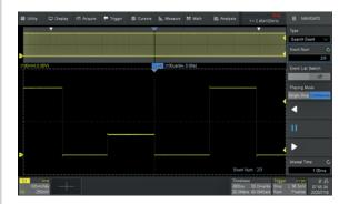
The T3DSO3000 can find events within an acquisition record or history acquisition based on user specified trigger conditions. Navigate browses through Events flagged by the Search, plays back history events or continuously moves the delay position on long records (useful in zoom view).
