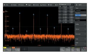
Two Math traces support Plus, Minus, Multiply, Divide, FFT, integration, differential, square root, average, Eres and formula editor, providing a quick insight into the waveform characteristics.
