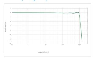
T3DSO31004 at 5 GSa/s shows exceptionally flat frequency response up to its maximum 1 GHz bandwidth.
