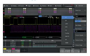
Trigger and decode up to 2 common embedded and automotive serial buses, I<sup>2</sup>C, SPI, UART, LIN, CAN, CAN FD, FlexRay, I<sup>2</sup>S, MIL-STD-1553B, SENT and Manchester. Protocol information can be quickly and intuitively displayed, time aligned with the waveform and in table format.
