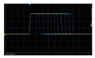
Segmented memory mode can store up to 100,000 waveforms into memory segments for capturing fast events in quick succession. Combine Sequence Mode with advanced triggers to isolate rare events. All the segments can be play back using the History function.
