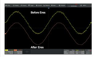
Enhanced Resolution (ERES) function reveals hidden waveform detail by using a linear average filter to reduce waveform noise on single acquisition waveforms, where regular averaging will not work. The ERES acquisition mode is hardware based, allowing waveforms to be captured at a faster rate.
