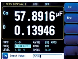
Continuous and Adjustable Frequency Freely Input Frequency Within Provided Frequency Range
