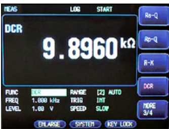
D.C. Resistance Measurement Ideal for inductive components' D.C. Characteristics Verification
