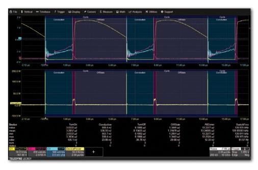
errors and the measurement parameters provide details of single cycle or average device power losses. Beyond the advanced power loss measurement capabilities, the Power Analyzer modulation analysis capabilities provide insight to understand control loop response to critical events such as a power supply's soft start performance or step response to line and load changes. The Line Power Analysis tool allows simple and quick pre-compliance testing to EN 61000-3-2.
