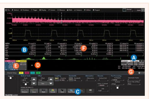
Channel, timebase, and trigger Α descriptors provide easy access to controls without navigating menus.
