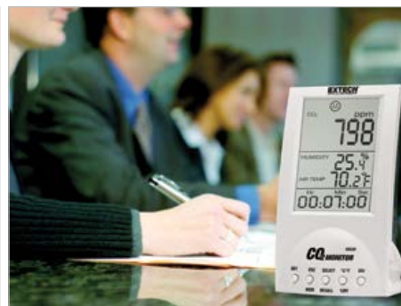
Six facial icons indicating CO 2 concentration level for indoor air quality.
