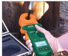
Verify resistance of cellular and communication tower ground grids
