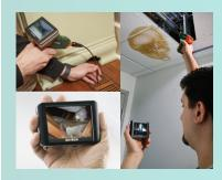
Extech's Video Borescope with a 5.2 mm diameter camera probe makes it possible to inspect hard to access areas through a small opening. It provides a glare-free close-up field of view. A color wireless monitor is included and can be detached from the base and viewed from a remote location up to 32 ft (9.75 m) away. Capture images/videos with date/time stamp and play back on the monitor or viewed on a PC.
