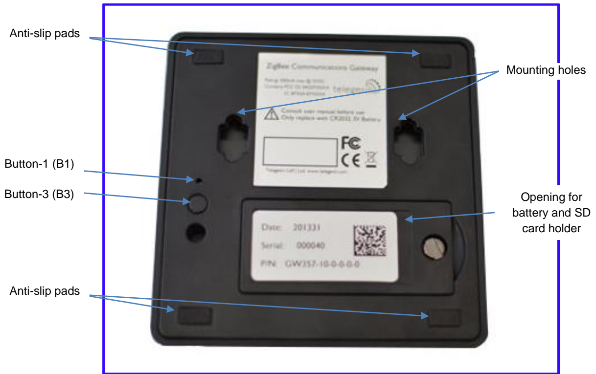
Figure 5: Gateway bottom view
