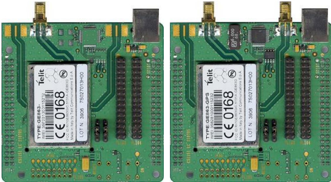
GE863 Interface Boards: GE863-QUAD or GE863-SIM (at left) and GE863-GPS (at right)
