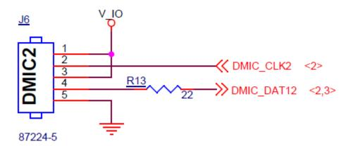
**Example DMIC Connector Signal Connections**
