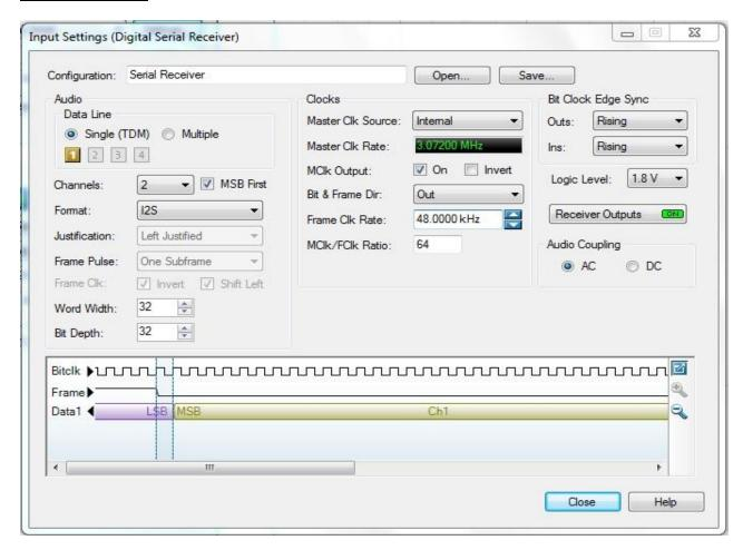
This figure shows an example of a typical timing configuration required to support I2S modes. Please note the SCLK and LRCLK relationship, and edge directions.
