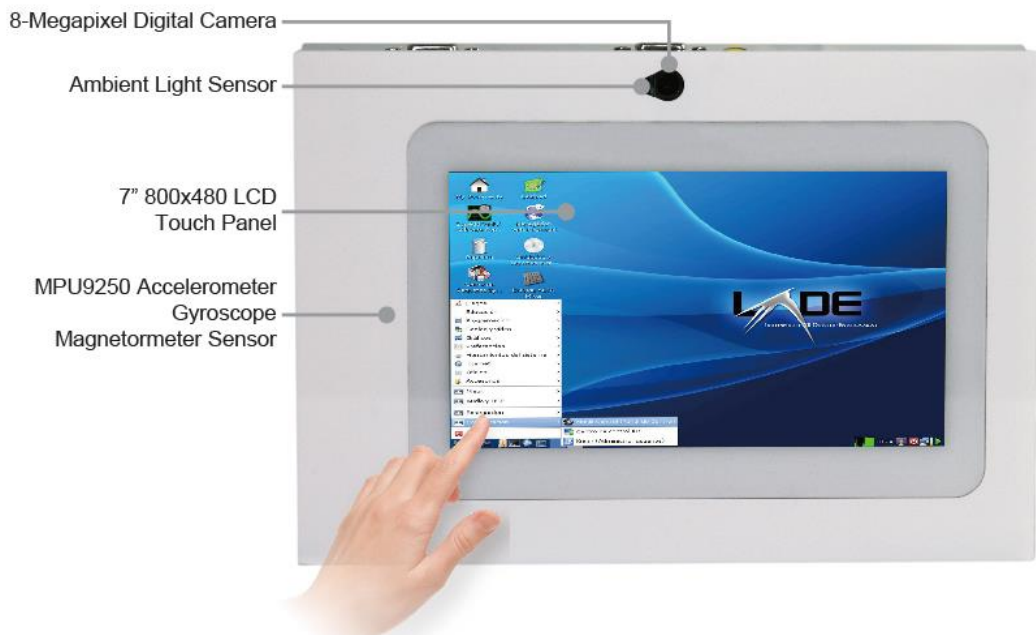
Figure 2-1 VEEK-MT2S (top view)
