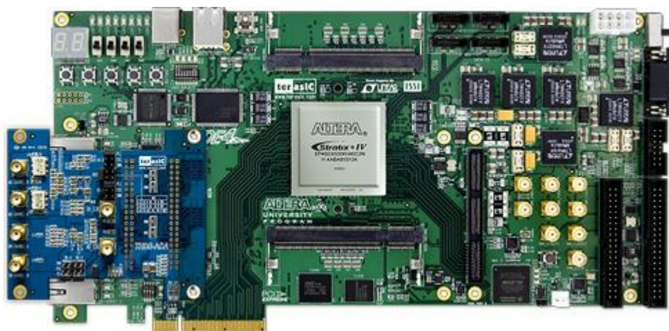
Figure 1-6 Connect ADA-HSMC with DE4 (HSMC port A)
