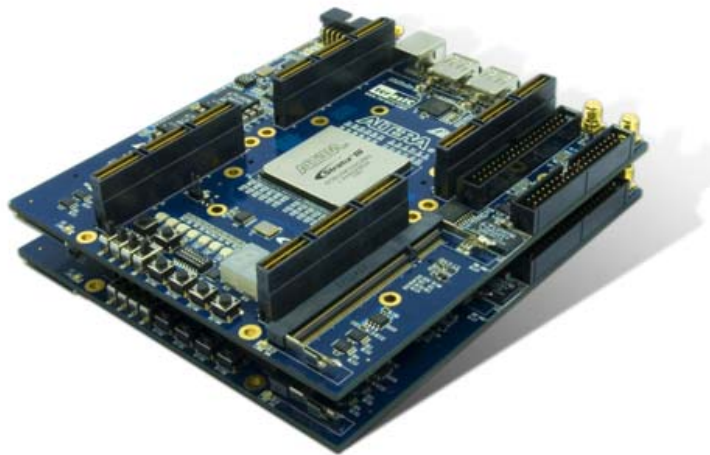
Figure 4.16. The connection of two DE3 boards
