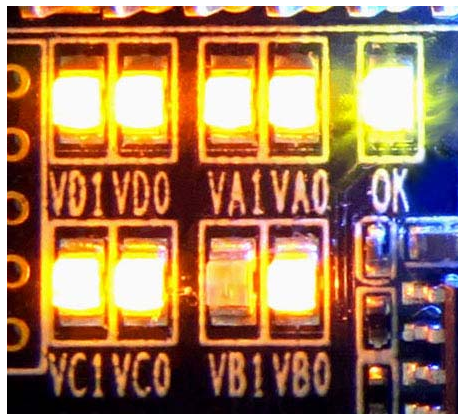
Figure 2.12a. Voltage-Level Indication for I/O Groups Example
