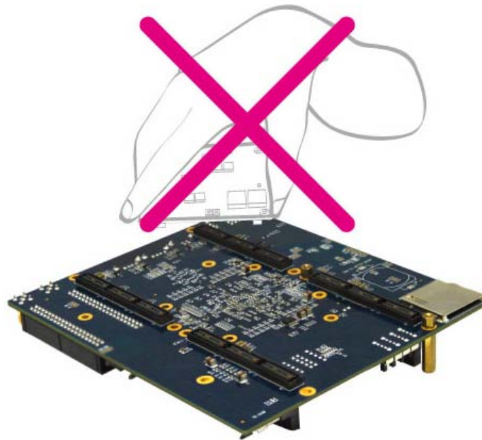
Figure 1.5 Do not install daughter cards to the back
