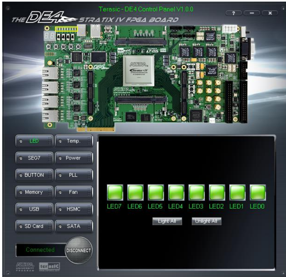
Figure 3–2 DE4 Control Panel is ready
