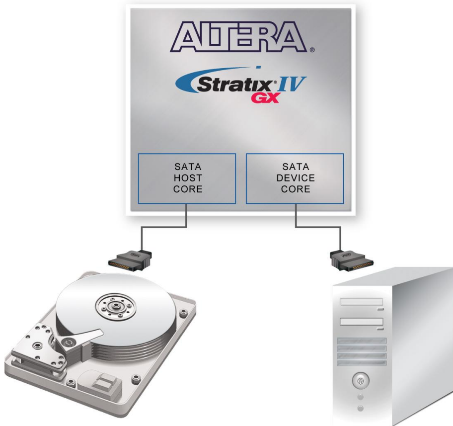
Figure 2–27 PC and storage device connection to the Stratix IV GX FPGA
