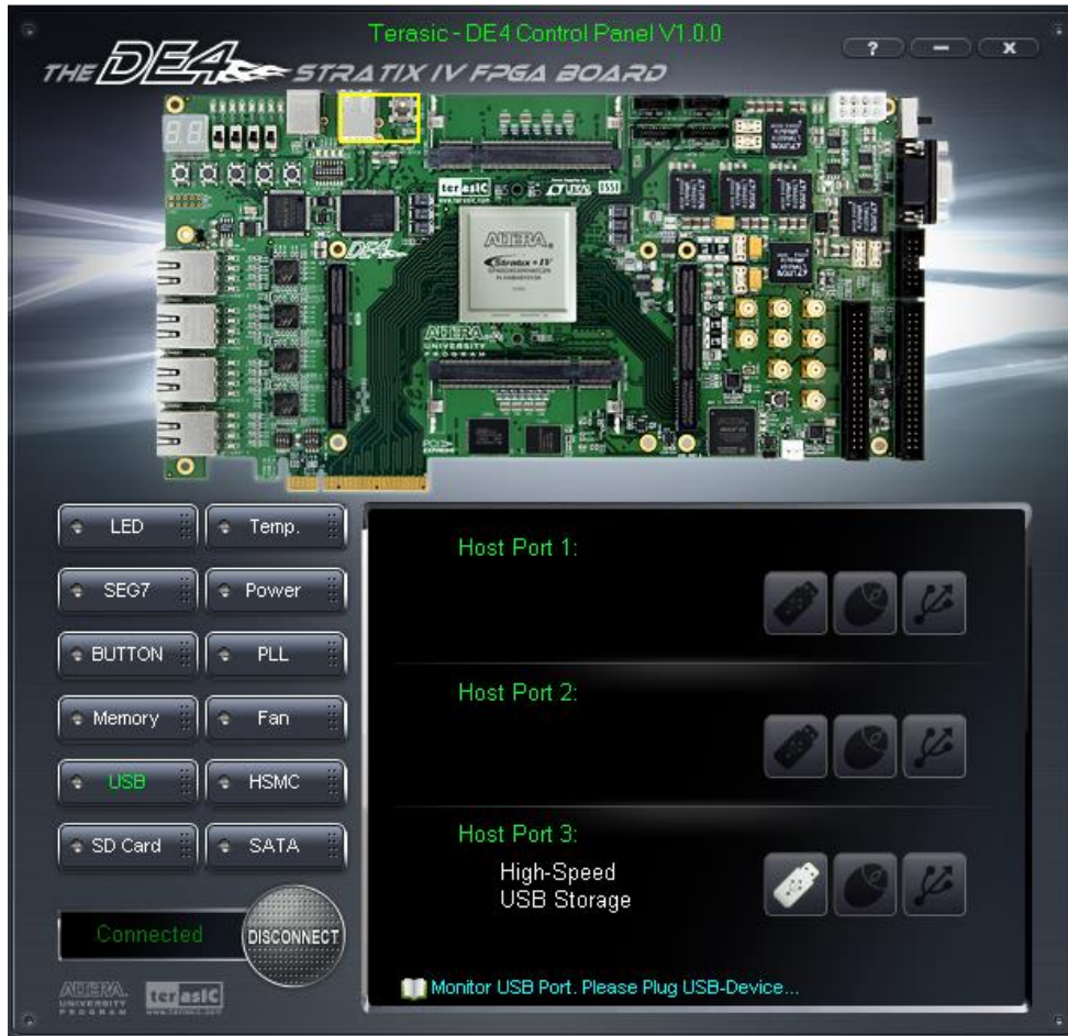
Figure 3–10 Monitoring status of USB ports
