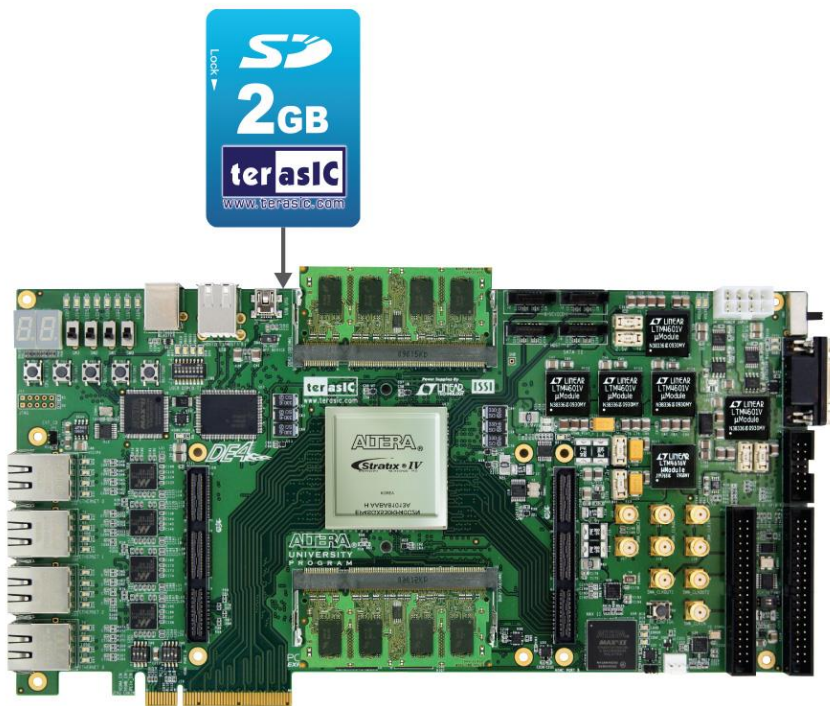
Figure 5–20 Insert SD Card for the SD-Card demonstration
