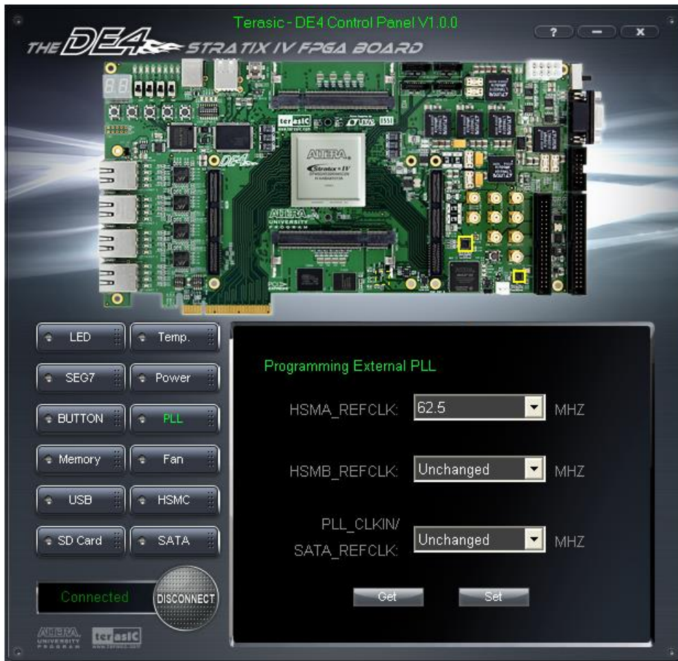
Figure 3–14 Programmable External PLL configured through Control Panel
