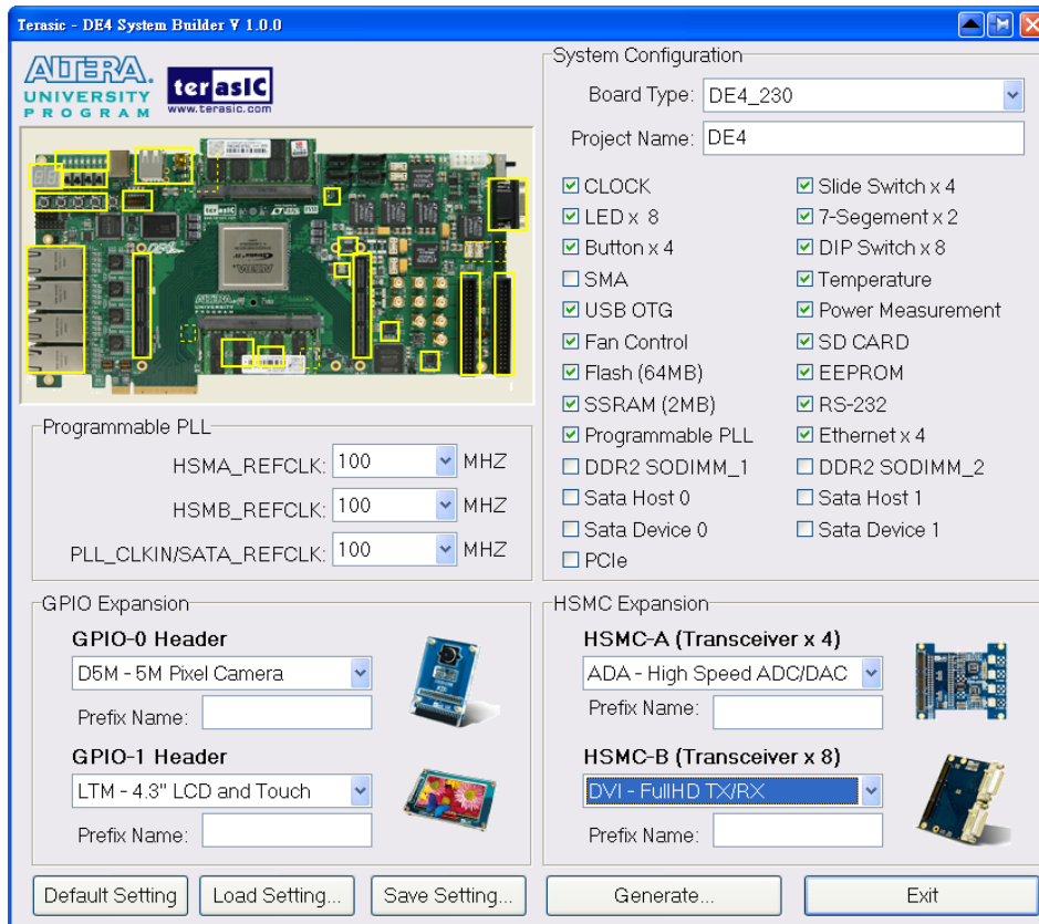
Figure 4–2 The DE4 System Builder window
