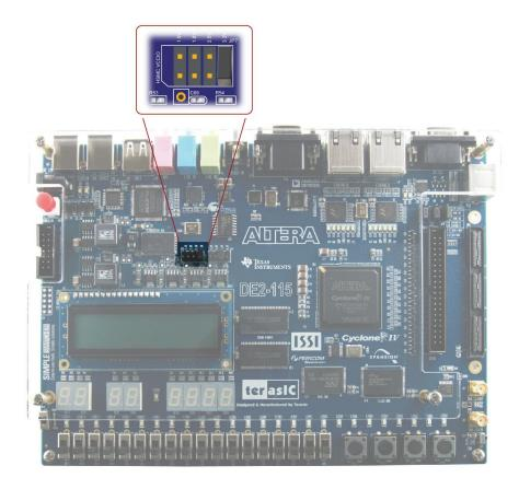
Figure 4-13 HSMC VCCIO supply voltage setting header
