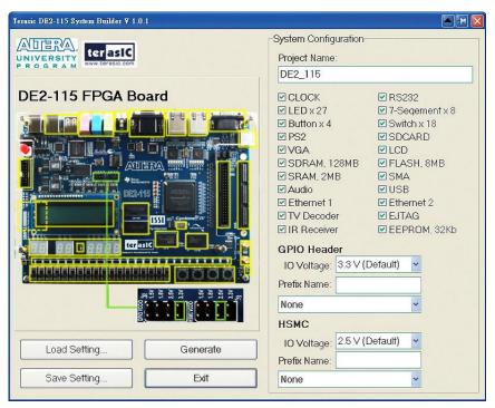
Figure 5-2 The DE2-115 System Builder window
