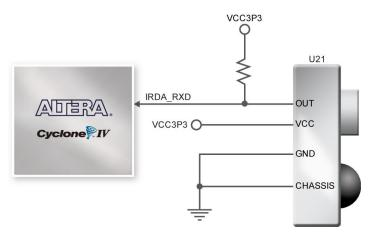
Figure 4-32 Connection between FPGA and IR
