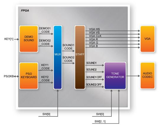
Figure 6-23 Block diagram of the Music Synthesizer design
