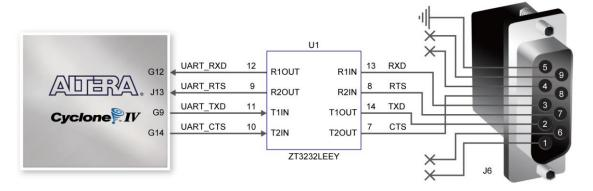
Figure 4-24 Connections between FPGA and ZT3232 (RS-232) chip
