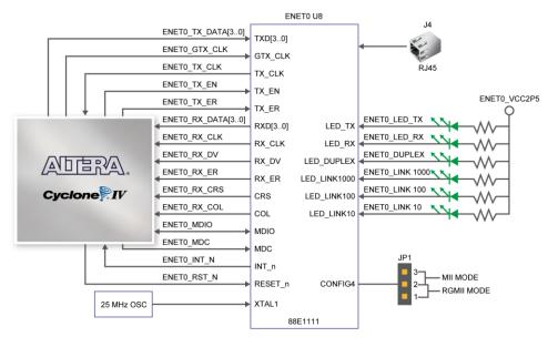
Figure 4-27 Connections between FPGA and Ethernet
