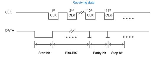
Figure 6-16 Waveforms on two lines while communication taking place
