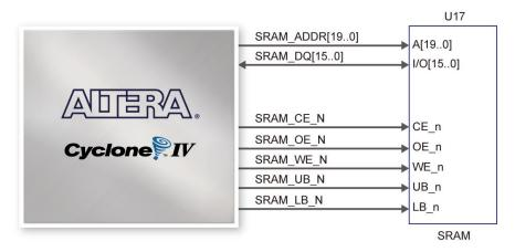
Figure 4-33 Connections between FPGA and SRAM
