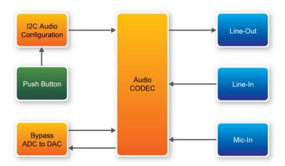
Figure 6-7 Block diagram of the Karaoke Machine demonstration
