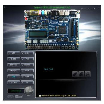
Figure 3-8 USB Mouse Monitoring Tool
