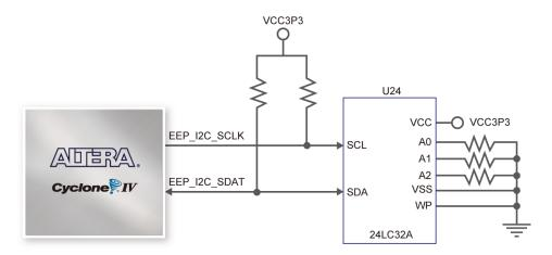
Figure 4-36 Connections between FPGA and EEPROM
