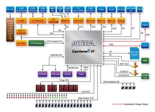
Figure 2-3 Block Diagram of DE2-115
