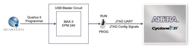
Figure 4-3 The JTAG configuration scheme
