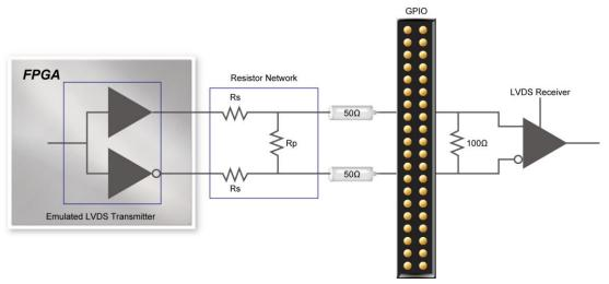
Figure 4-19 Using Emulated LVDS on GPIO
