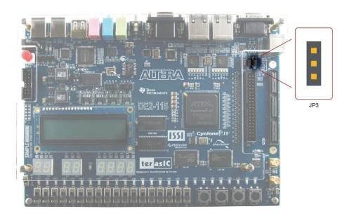
Figure 4-2 The JTAG chain configuration header
