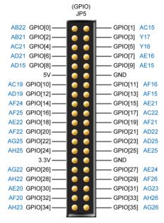
Figure 4-15 GPIO Pin Arrangement
