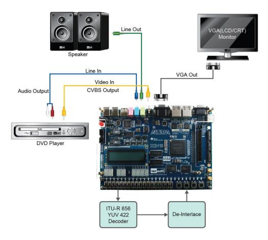
Figure 6-2 The setup for the TV box demonstration
