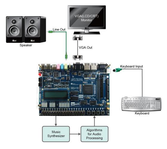
Figure 6-24 The Setup of the Music Synthesizer Demonstration
