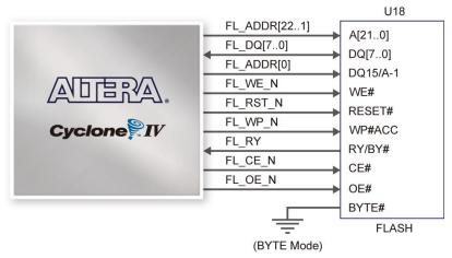
Figure 4-35 Connections between FPGA and Flash
