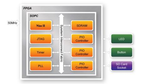
Figure 6-9 Block Diagram of the SD Card Demonstration
