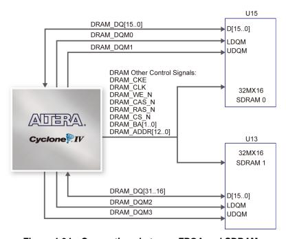
Figure 4-34 Connections between FPGA and SDRAM
