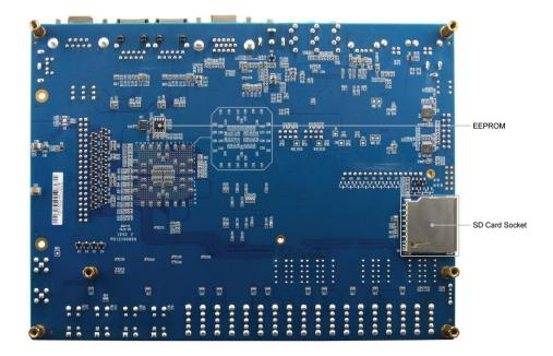
Figure 2-2 The DE2-115 board (bottom view)
