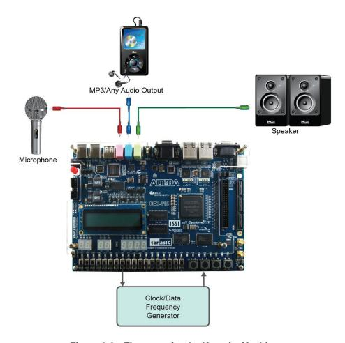
Figure 6-8 The setup for the Karaoke Machine
