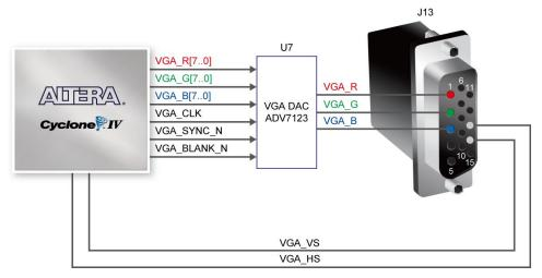
Figure 4-21 Connections between FPGA and VGA
