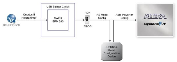
Figure 4-5 The AS configuration scheme
