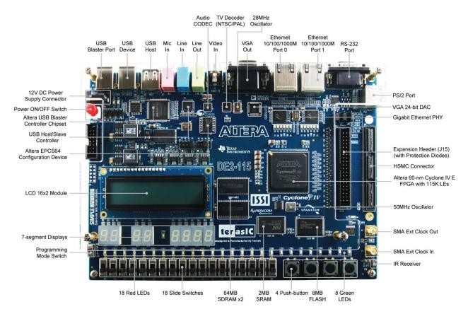
Figure 2-1 The DE2-115 board (top view)
