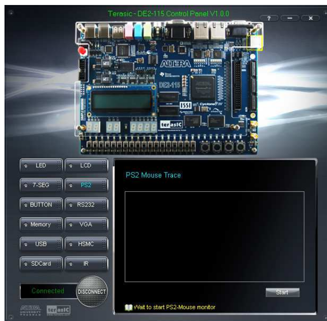
Figure 3-9 PS/2 Mouse Monitoring Tool
