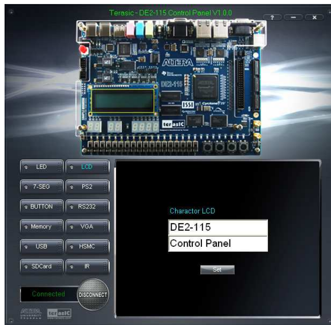
Figure 3-5 Controlling the LCD display
