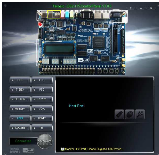
Figure 3-8 USB Mouse Monitoring Tool
