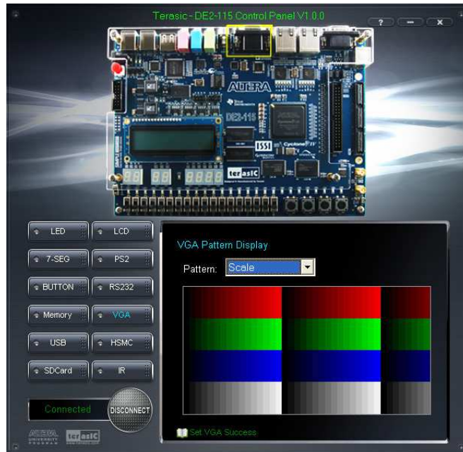
Figure 3-12 Controlling VGA display
