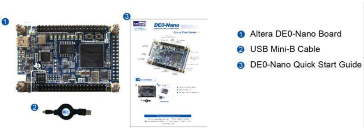
Figure 1-2 DE0-Nano kit package contents
