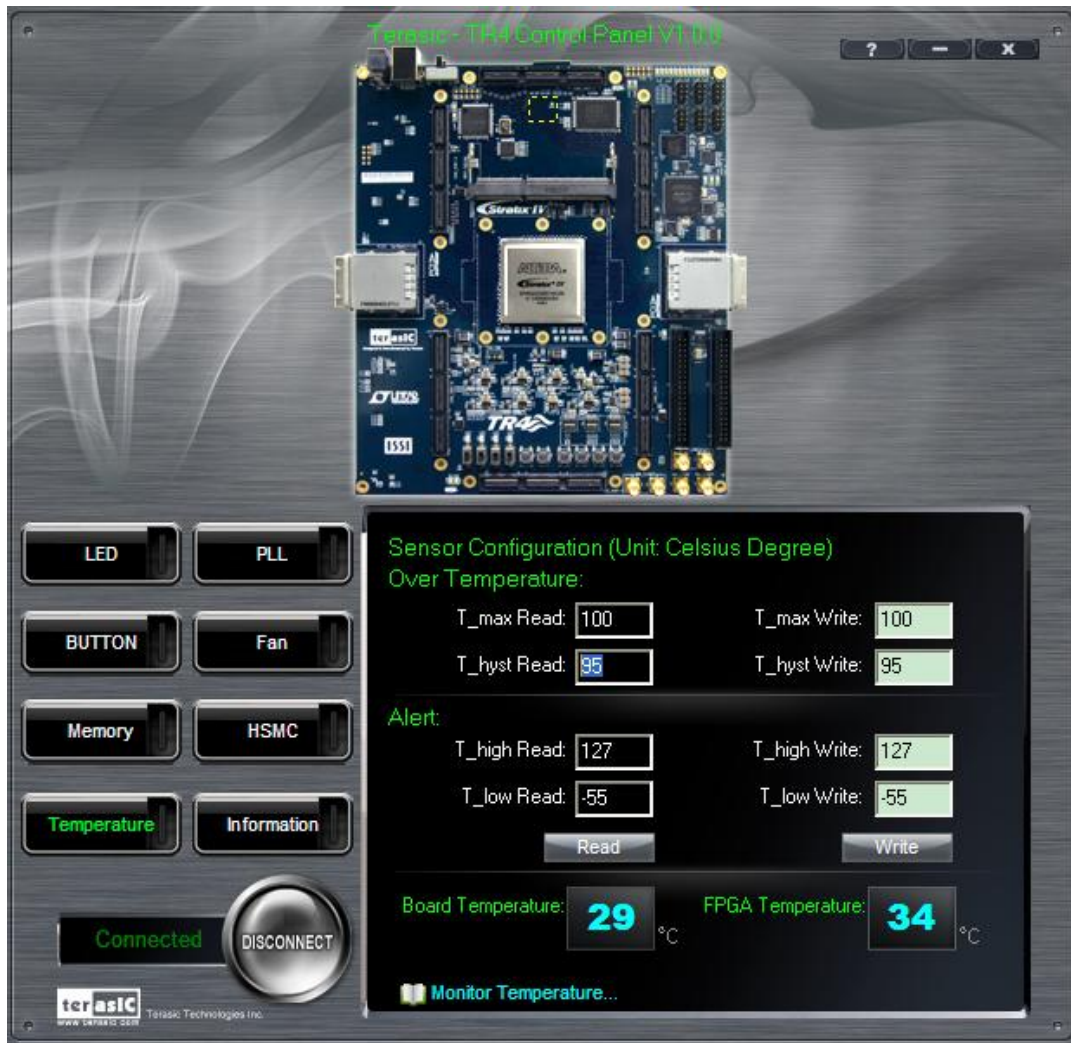
Figure 3-9 Accessing the Temperature Sensor through Control Panel
