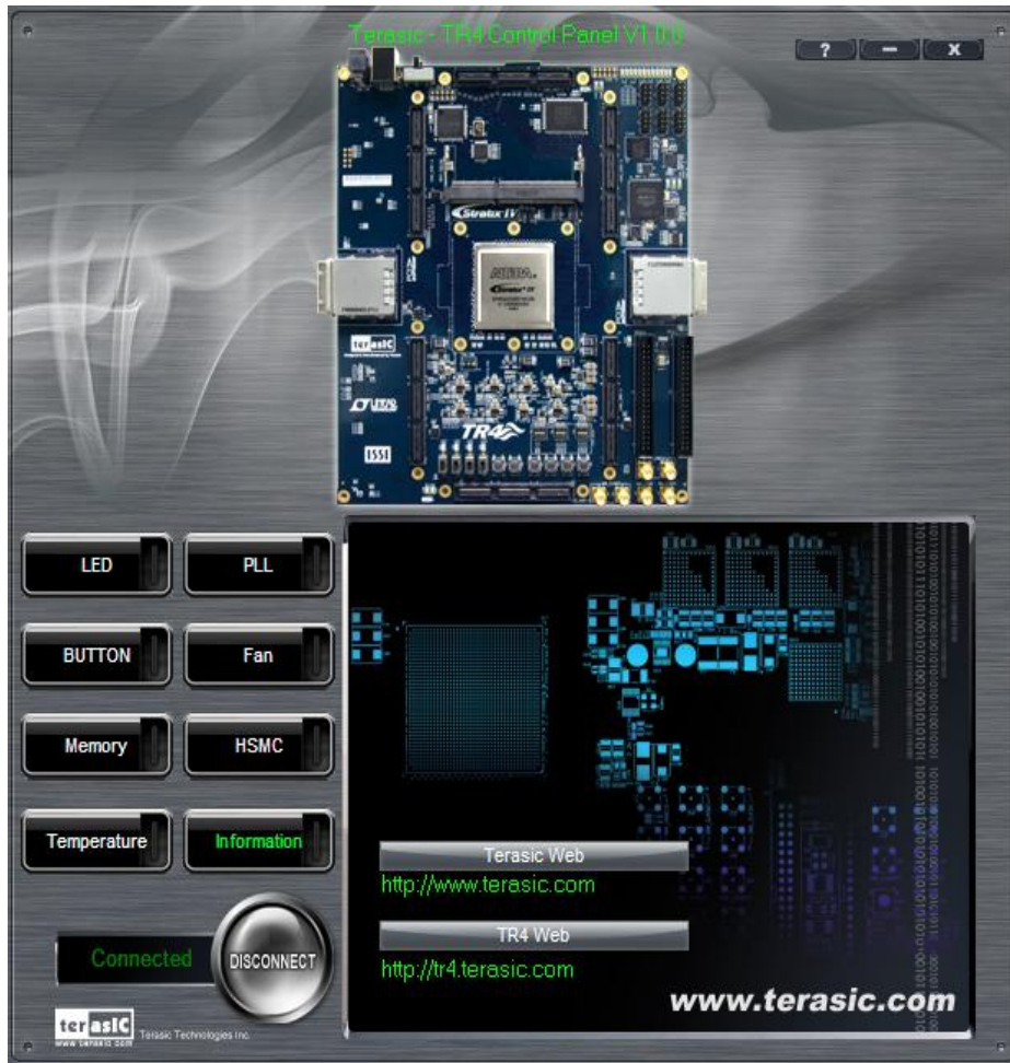
Figure 3-13 Information Tab of TR4 Control Panel
