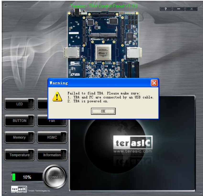
Figure 3-3 The TR4 Control Panel Fails to Download .sof File
