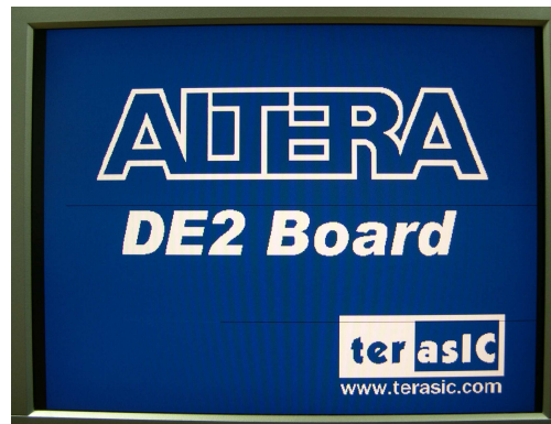
Figure 2.3. The default VGA output pattern.
