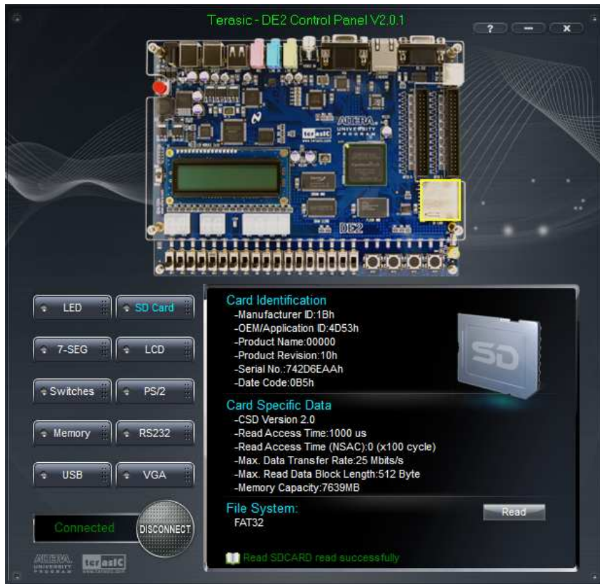
Figure 3.10. Reading the SD Card Identification and Specification.
