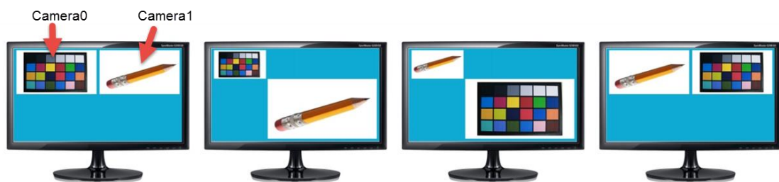
Figure 5-6 Four display modes in Mixer function.
