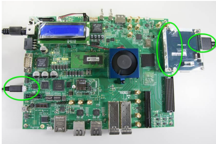
Figure 5-8 Setup A10SoC_D8M_FMC_VIP demonstration
