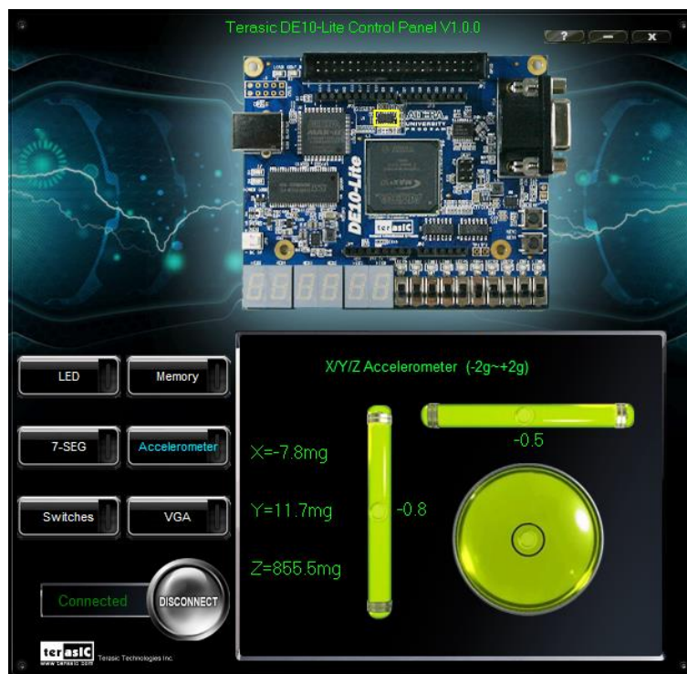
Figure 2-7 Level by G-Sensor
