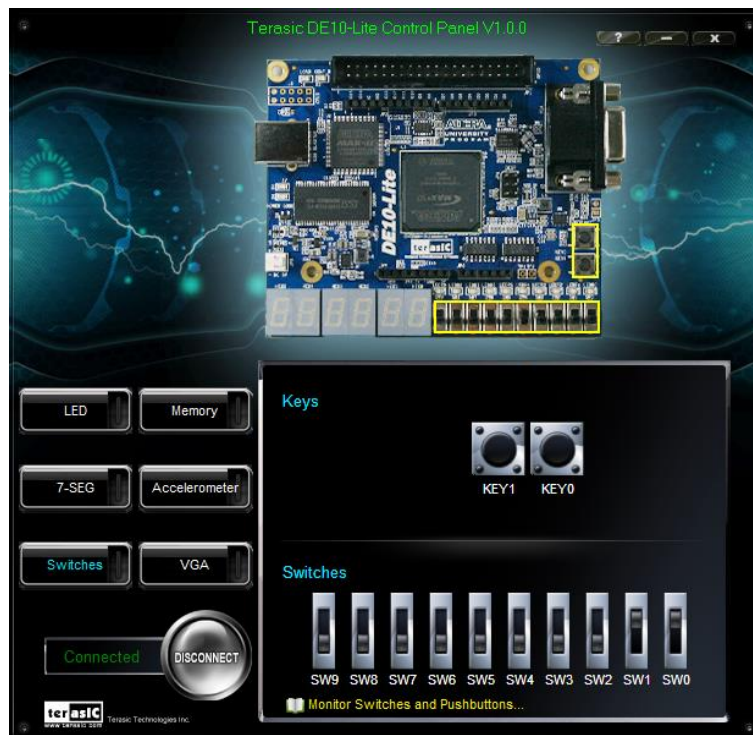
Figure 2-5 Monitoring switches and buttons
