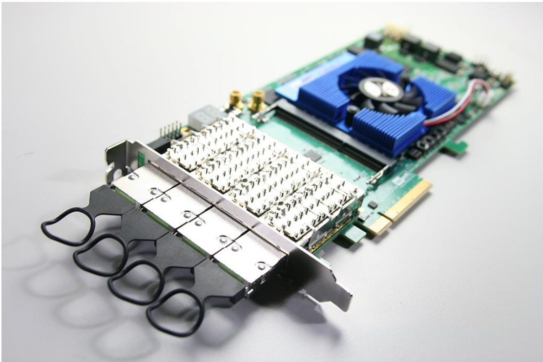
Figure 9-4 Four QSFP+ Loopback Fixtures Installed
