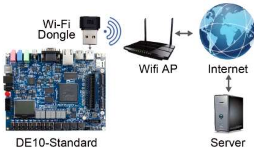
Figure 6-15 System diagram of USB Wi-Fi dongle
