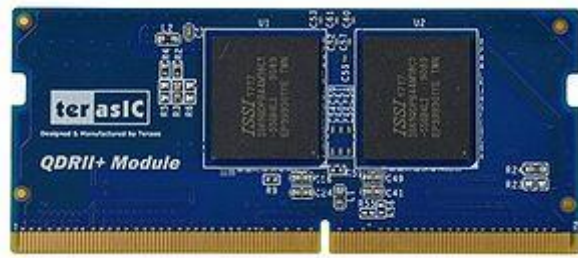
Figure 4-18 Terasic QDRII+ module with DDR4 SO-DIMM interface
