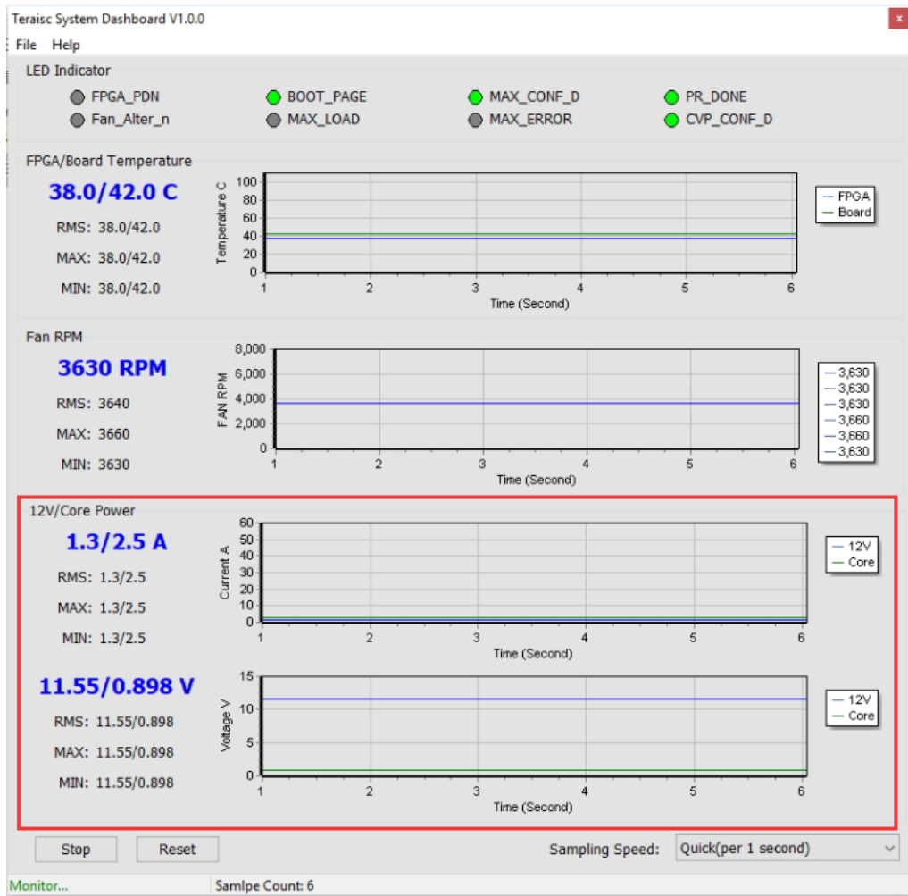
Figure 8-21 Power Monitor Section
