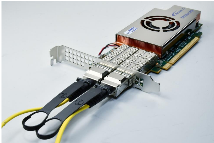
Figure 7-3 One QSFP+ Cables Installed
