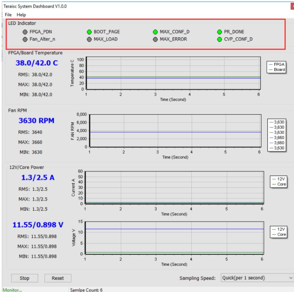
Figure 8-18 FPGA Status section
