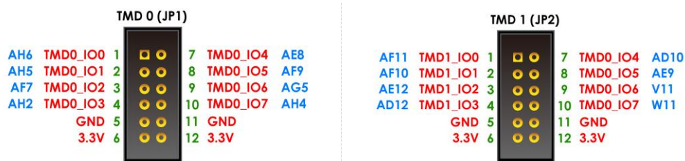
Figure 5-5 TMD Pin Arrangement
