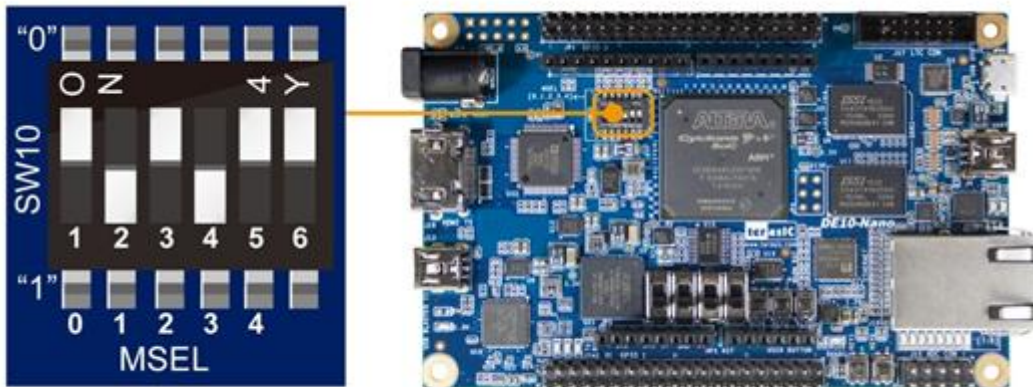
Figure 7-3 Set MSEL[4:0] to "01010" for ARM Version Mode
