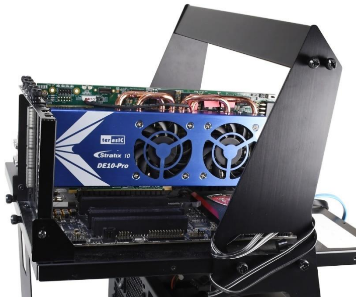
Figure 8-4 FPGA board installation on PC
