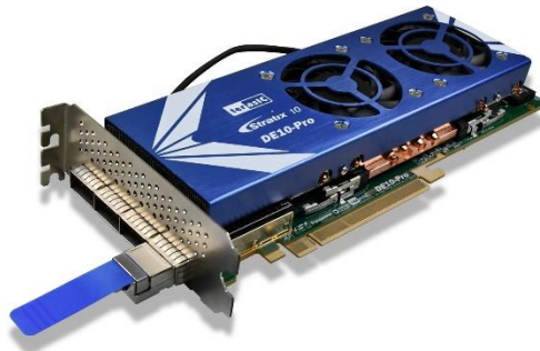
Figure 9-7 Setup QSFP28 loopback fixture
