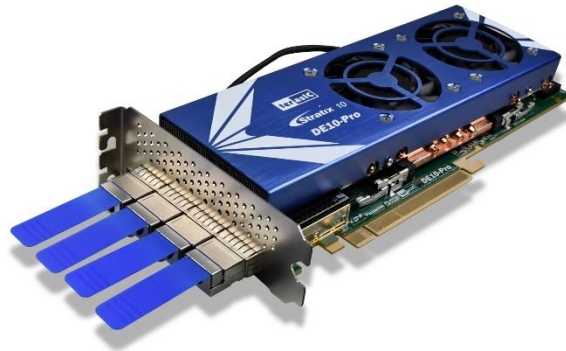
Figure 9-2 QSFP28 Transceiver Loopback Test in Progress
