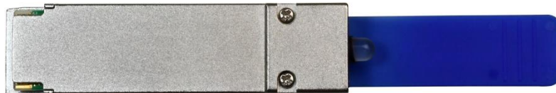
Figure 6-1 QSFP28 Loopback fixtures
