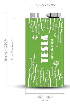
**DESCRIPTION:** Nickel Metal Hydride Rechargeable Battery, 9V Size **CHEMICAL SYSTEM:** Nickel Metal Hydride SHELF LIFE: Guaranteed for 500 recharges **NOMINAL VOLTAGE:** 8,4 Volts NOMINAL DIMENSIONS: 26.5(L)mm × 17.5(W)mm × 48.5(H)mm **TERMINALS:** Nickel plated miniature snap fasteners JACKET: Foil jacket **APPLICATIONS:** All electronics devices e.g. toys, microphones, smoke detectors, photographic equipment. **STORAGE TEMPERATURE:** -20 °C to + 35 °C **NOMINAL WEIGHT:** 46,5 g
