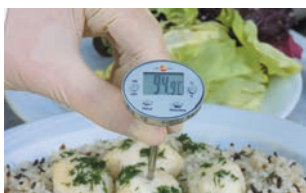
For temperature spot-check measurements in food production
