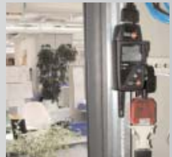
Read out the data stored in the logger via the PC network using the Ethernet adapter
