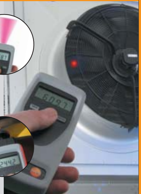
Rpm measurement on rotating parts, non-contact and mechanical
