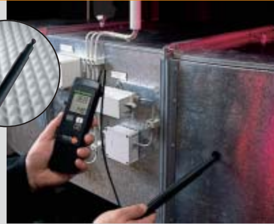
Measuring the flow speed in a ventilation duct
