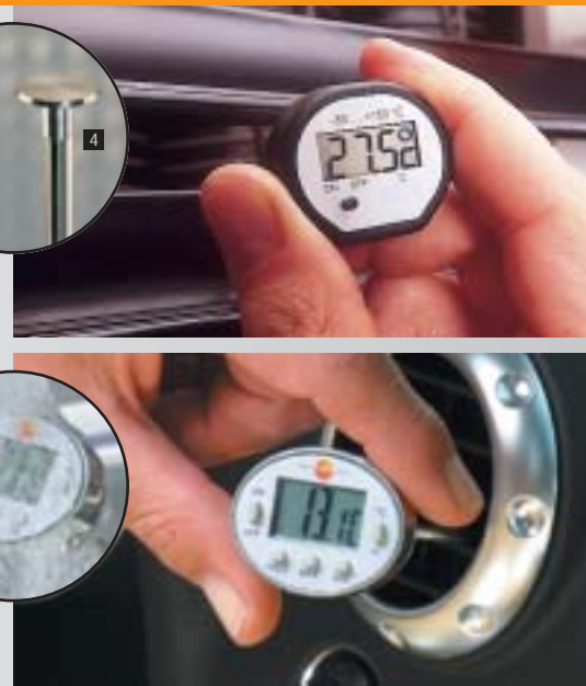
Measurements in air conditioning units
