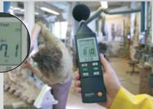
testo 816, Checking noise control
