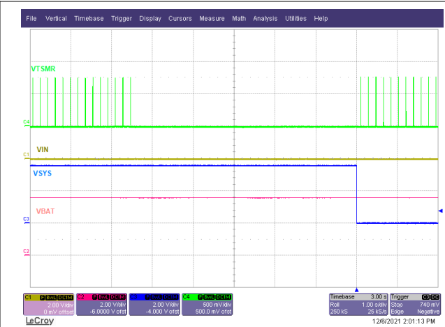
Figure 9-7. Enter Shipmode with Push Button Long Press
