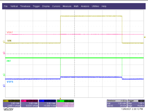
Figure 9-11. Power Good Interrupt on /INT
