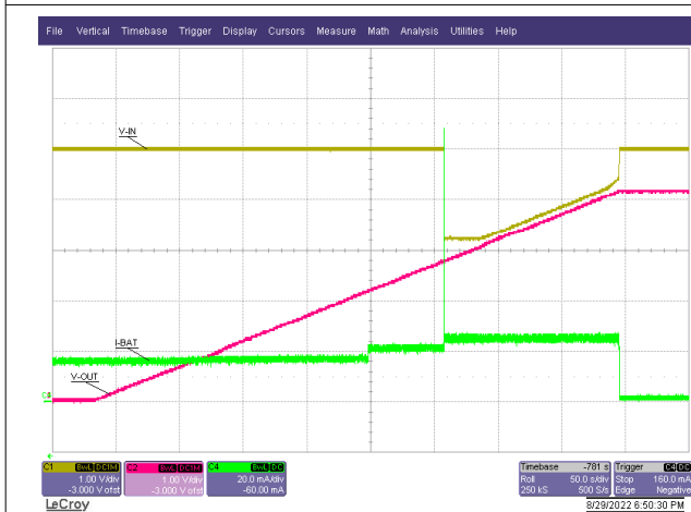
R_{ISET} = 1.5\text{ k}\Omega V_{SET} = 4.2\text{ V} Input source I_{limit} = 25\text{ mA}
