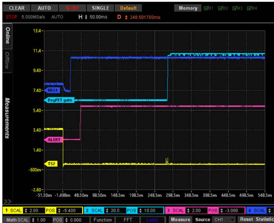
图 16-5. Startup Sequence Using [FASTADC] = 1 , with the [INITCOMP] Flag Displayed on the ALERT Pin.
