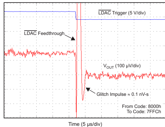
Figure 80. Glitch Impulse, Falling Edge, 1-LSB Step
