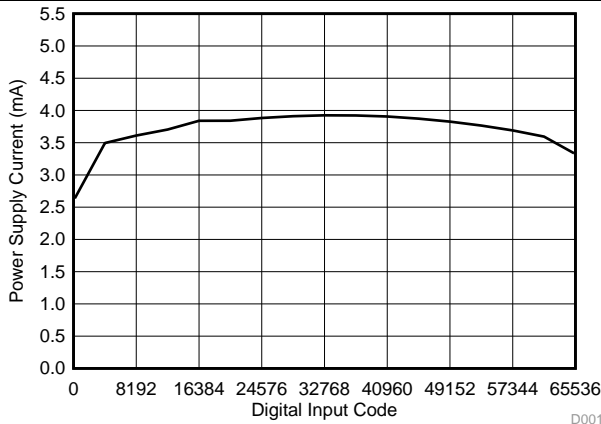
Figure 33. Power Supply Current vs Digital Input Code
