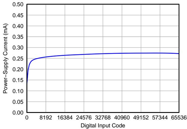
Figure 51. Power-Supply Current vs Digital Input Code
