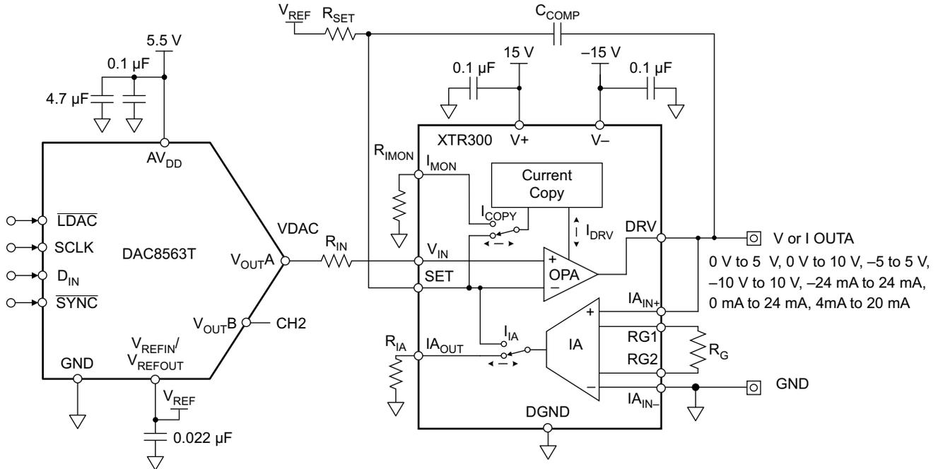
Figure 96. DAC8563T and XTR300 Discrete Analog Output Module
