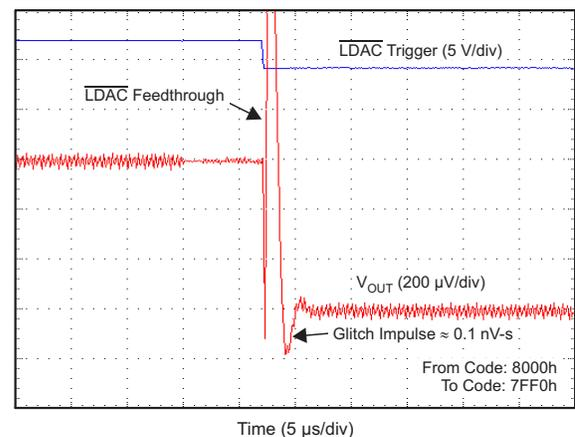
**Figure 84. Glitch Impulse, Falling Edge, 16-LSB Step**
