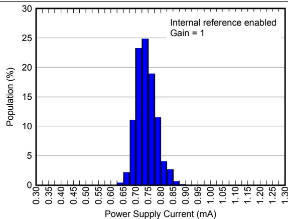
Figure 72. Power-Supply Current Histogram
