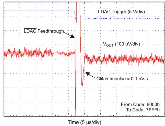
**Figure 80. Glitch Impulse, Falling Edge, 1-LSB Step**
