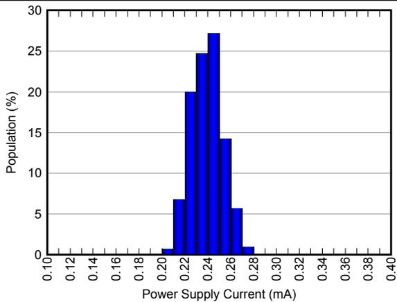
Figure 53. Power-Supply Current Histogram
