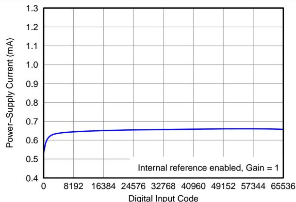
Figure 70. Power-Supply Current vs Digital Input Code
