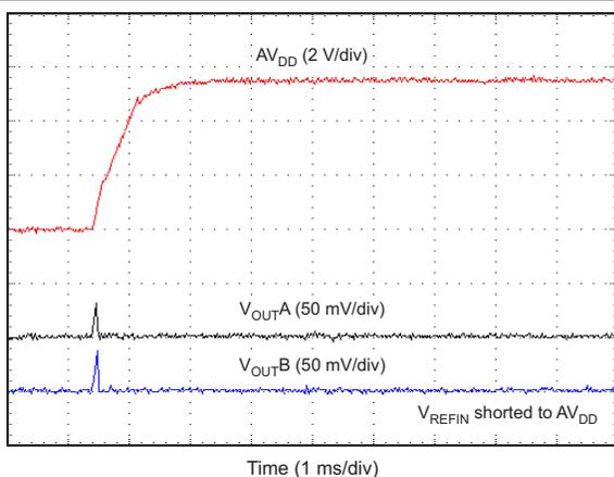
**Figure 35. Power-On Glitch, Reset to Zero Scale**
