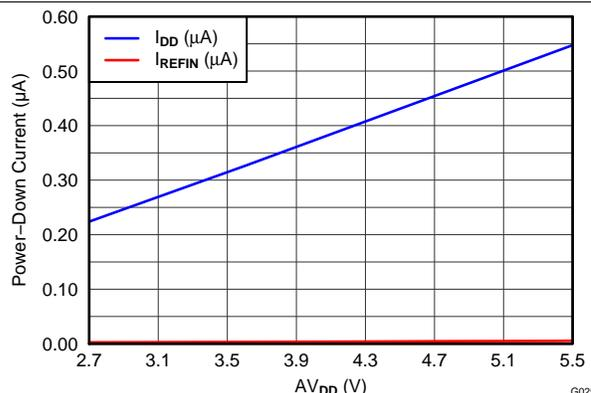
Figure 29. Power-Down Current vs Power-Supply Voltage
