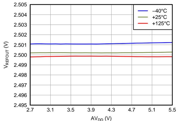
Figure 7. Internal Reference Voltage vs Supply Voltage
