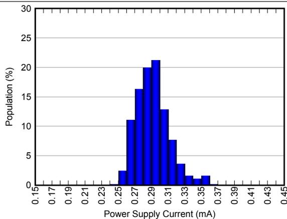
Figure 24. Power-Supply Current Histogram
