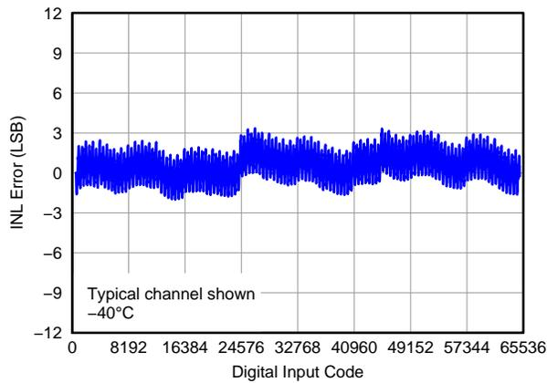
Figure 8. Linearity Error vs Digital Input Code ( $-40^\circ\text{C}$ )
