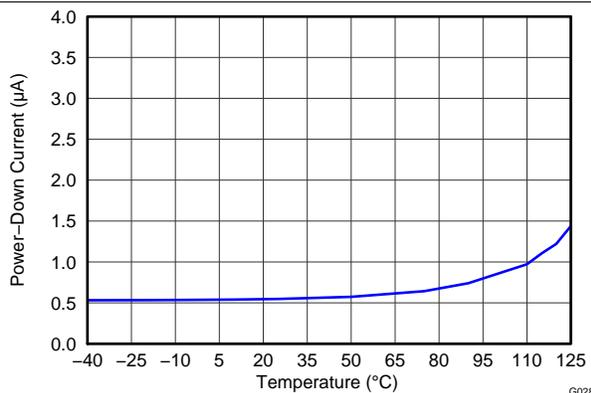
Figure 28. Power-Down Current vs Temperature
