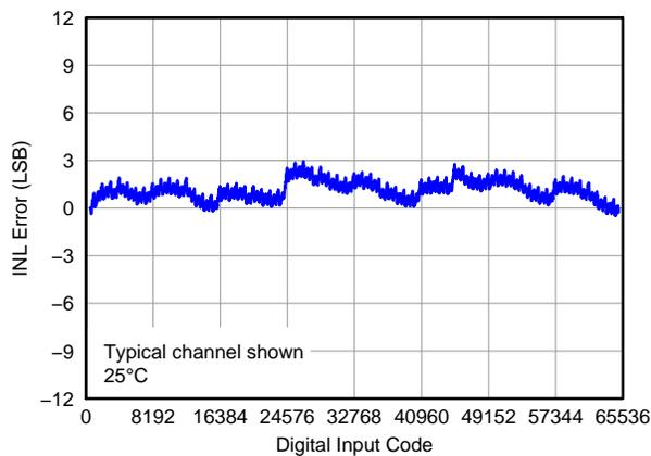
Figure 57. Linearity Error vs Digital Input Code ( $25^\circ\text{C}$ )
