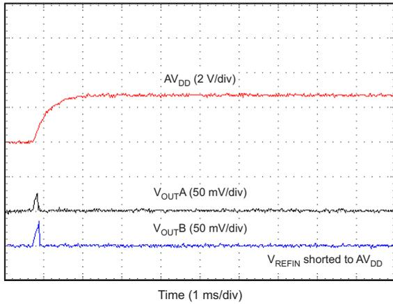
**Figure 85. Power-On Glitch, Reset to Zero Scale**
