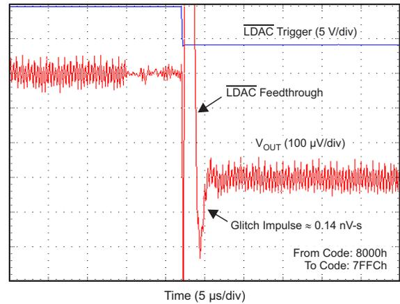
Figure 40. Glitch Impulse, Falling Edge, 4-LSB Step
