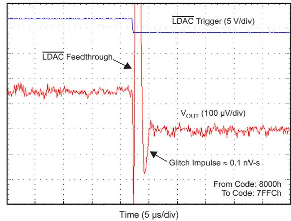
**Figure 82. Glitch Impulse, Falling Edge, 4-LSB Step**
