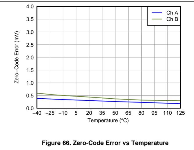
Typical Characteristics: DAC at  $V_{DD} = 2.7\text{ V}$  (continued)
