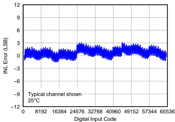
Figure 10. Linearity Error vs Digital Input Code ( $25^\circ\text{C}$ )
