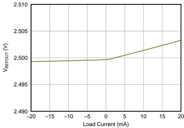
Figure 4. Internal Reference Voltage vs Load Current
