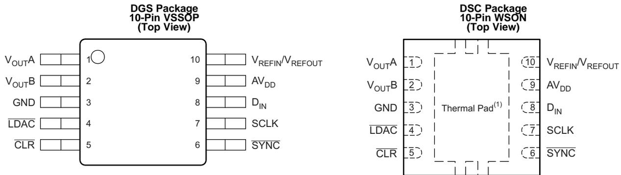
(1) TI recommends connecting the thermal pad to the ground plane for better thermal dissipation.
