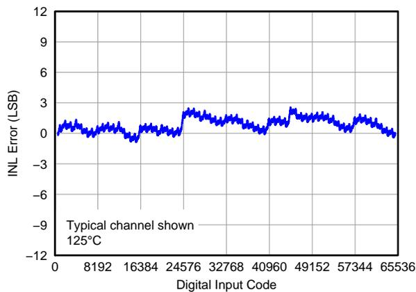
Figure 59. Linearity Error vs Digital Input Code ( $125^\circ\text{C}$ )
