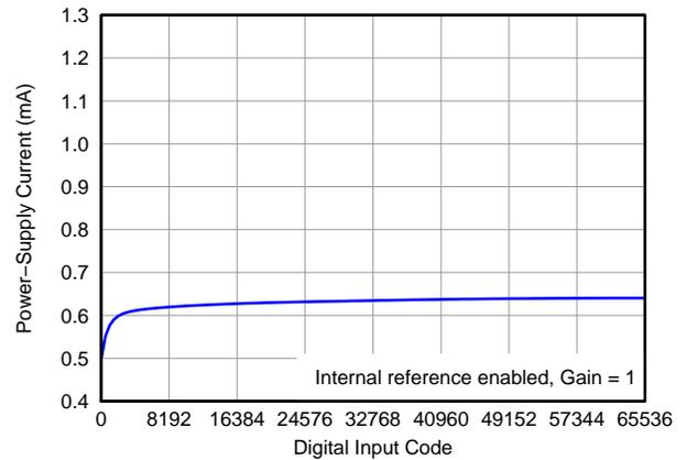
Figure 52. Power-Supply Current vs Digital Input Code
