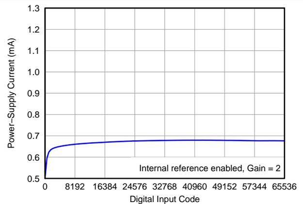
Figure 23. Power-Supply Current vs Digital Input Code
