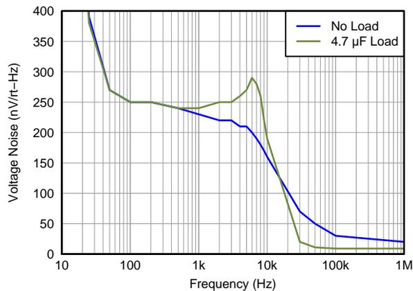
Figure 6. Internal Reference Noise Density vs Frequency
