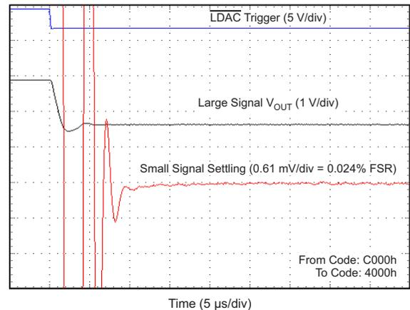
Figure 78. Half-Scale Settling Time, Falling Edge
