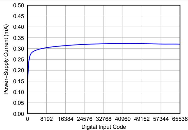
Figure 22. Power-Supply Current vs Digital Input Code
