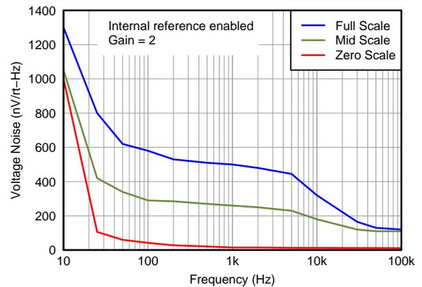
**Figure 46. DAC Output Noise Density vs Frequency**
