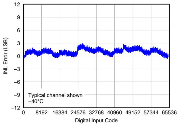
Figure 55. Linearity Error vs Digital Input Code ( $-40^\circ\text{C}$ )
