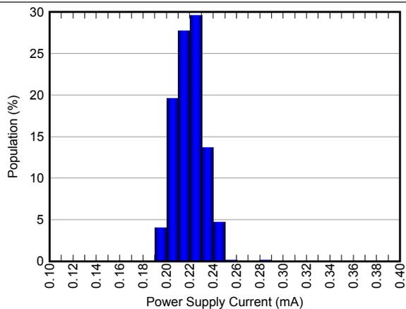
Figure 71. Power-Supply Current Histogram
