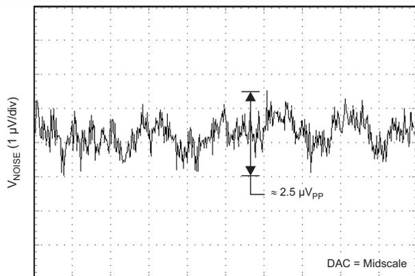
**Figure 47. DAC Output Noise, 0.1 Hz to 10 Hz**
