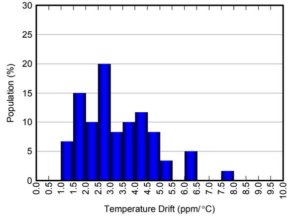
Figure 3. Internal Reference Voltage, Temperature Drift Histogram
