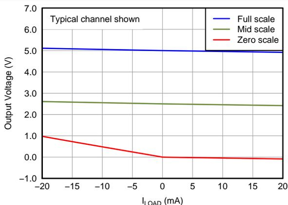
Figure 30. DAC Output Voltage vs Load Current
