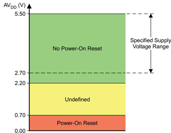
**Figure 91. Relevant Voltage Levels for POR Circuit**
