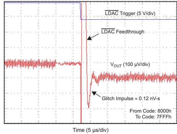
Figure 38. Glitch Impulse, Falling Edge, 1-LSB Step
