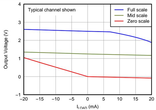
Figure 74. DAC Output Voltage vs Load Current
