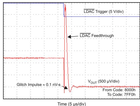
Figure 42. Glitch Impulse, Falling Edge, 16-LSB Step
