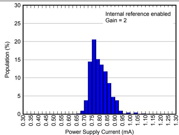
Figure 25. Power-Supply Current Histogram
