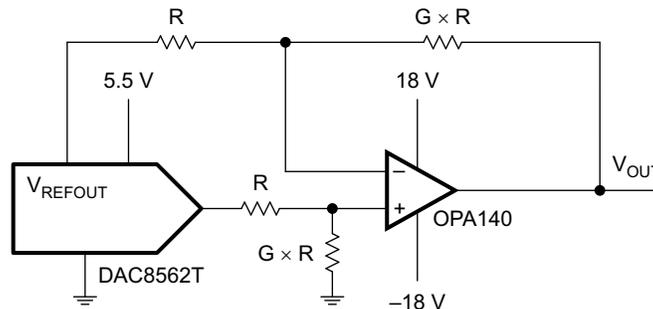
**Figure 99. Bipolar Output Range Circuit Using DAC8562T**
