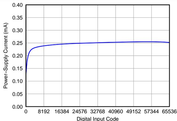
Figure 69. Power-Supply Current vs Digital Input Code
