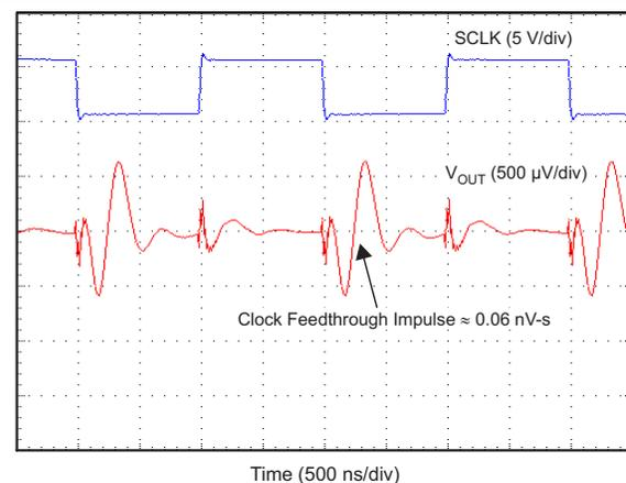
**Figure 48. Clock Feedthrough, 500 kHz, Midscale**
