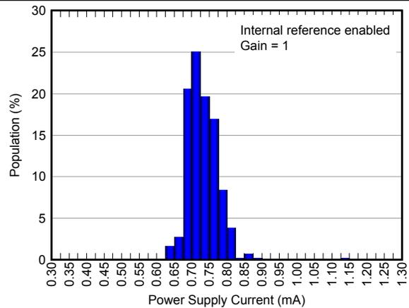
Figure 54. Power-Supply Current Histogram
