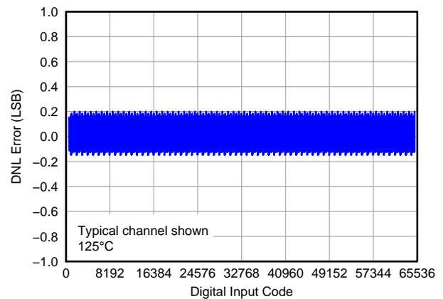
Figure 13. Differential Linearity Error vs Digital Input Code ( $125^\circ\text{C}$ )
