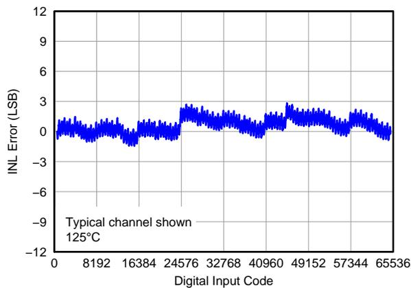
Figure 12. Linearity Error vs Digital Input Code ( $125^\circ\text{C}$ )
