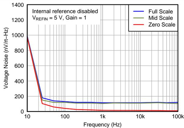
**Figure 45. DAC Output Noise Density vs Frequency**
