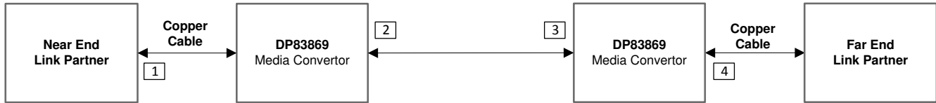
图 9-12. Link Loss Pass-Through
