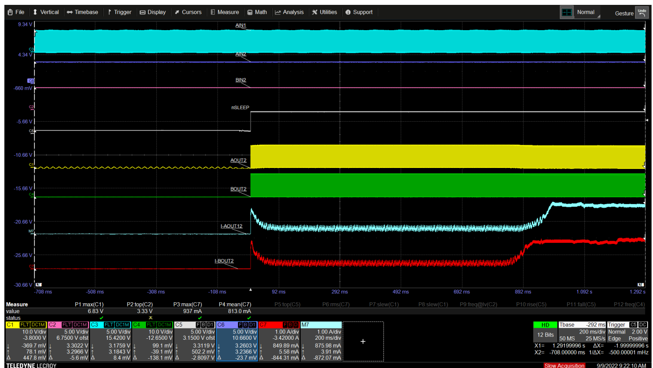
Figure 10-9. No Current Regulation
