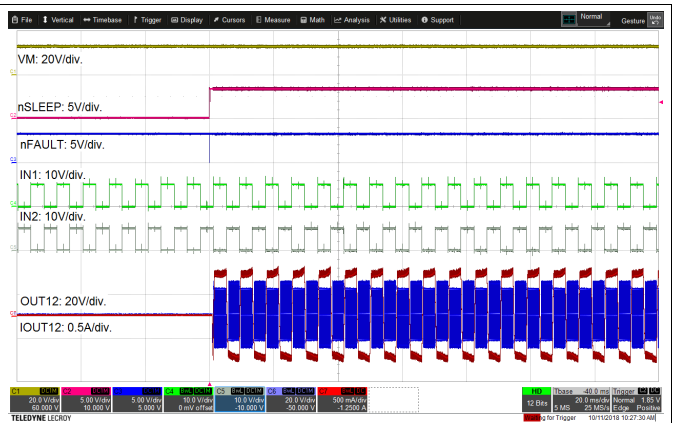
图 47. Device Power-up with nSLEEP
