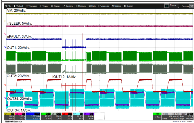
图 54. Undervoltage Lockout Operation
