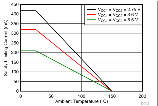
Figure 2. Thermal Derating Curve for Safety Limiting Current for DBQ-16 Package
