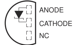
1.2 V ... LP (TO-92/TO-226) PACKAGE (TOP VIEW)
