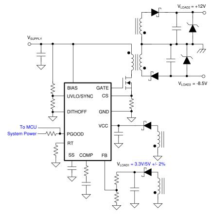
图 10-11. Primary-Side Regulated Multiple-Output Isolated Flyback
