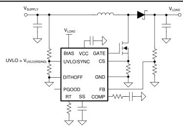
图 9-6. Decrease the Minimum Operating Voltage After Start-Up
