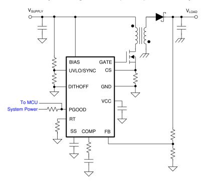
图 10-12. Typical Non-Isolated Flyback
