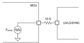
图 9-16. Shutdown and Clock Synchronization
