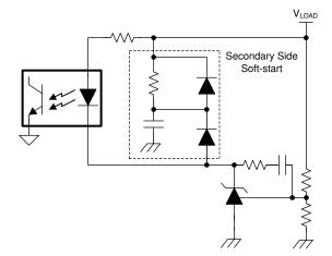
图 9-9. Secondary-Side Soft Start in Flyback
