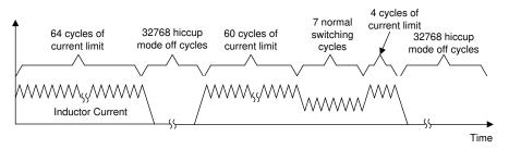
图 9-21. Hiccup Mode Overload Protection
