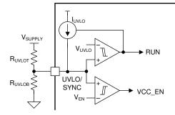
图 9-1. Line UVLO and Enable
