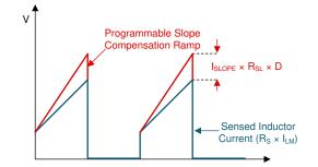
图 9-20. Slope Compensation Ramp (b) at Current Limit Comparator Input
