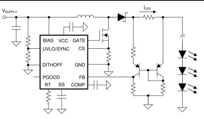
图 10-13. LED Driver with High-Side Current Sensing
