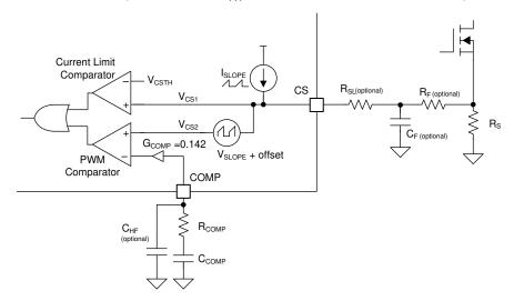
图 9-18. Current Sensing and Slope Compensation
