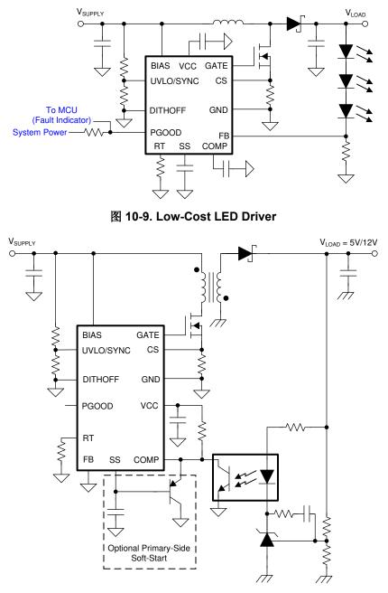
图 10-10. Secondary-Side Regulated Isolated Flyback
