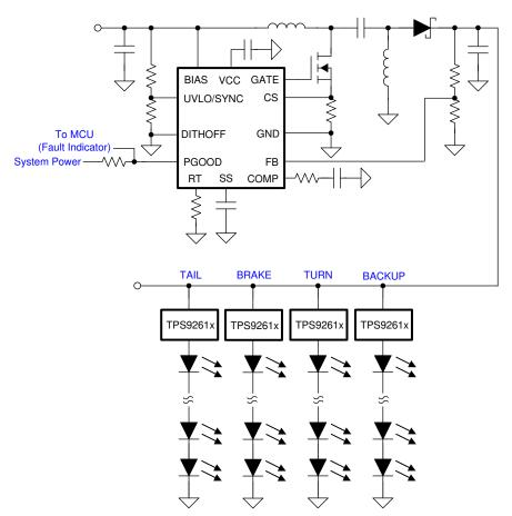
图 10-14. Dual-Stage Automotive Rear-Lights LED Driver
