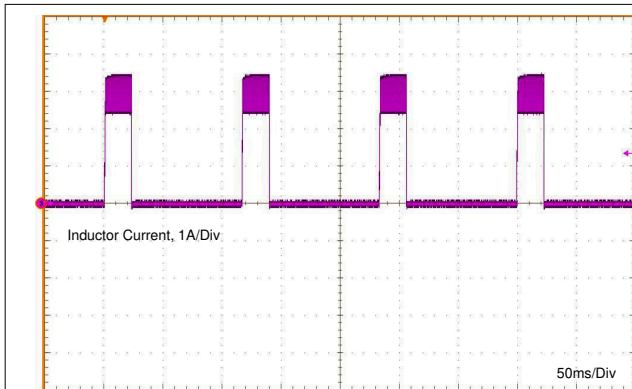
图 8-5. Inductor Current Burst in Short-Circuit Mode
