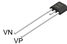
LPG Package 2-Pin TO-92 Top View
