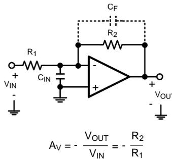
**Figure 46. Inverting Amplifier**
