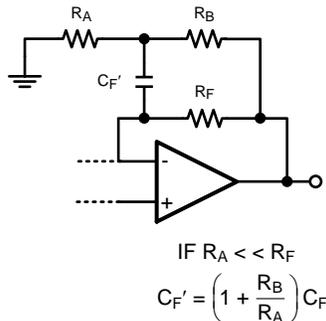
Figure 54. Obtaining Small  $C_F$  from Large  $C_{F'}$
