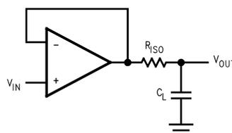
**Figure 45. Isolation of  $C_L$  to Improve Stability**
