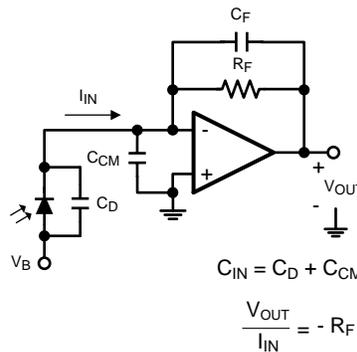
Figure 52. Photodiode Transimpedance Amplifier
