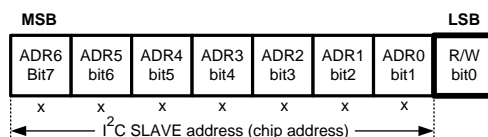
Figure 23. I 2 C Chip Address
