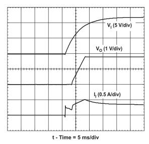
Figure 11. Power-Up Waveforms
