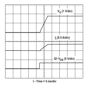
Figure 13. Power-Up Response From Inhibit Control
