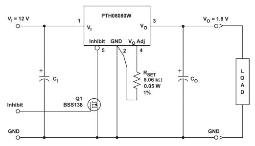
Figure 12. On/Off Inhibit Control Circuit
