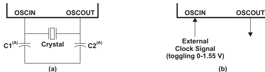
Figure 5-3. Recommended Crystal/Clock Connection
